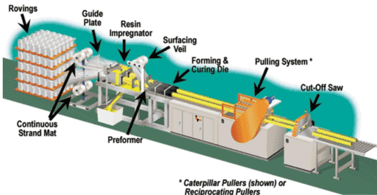
**a) Material In-Feed :** Reinforcements are to be in a package designed for continuous feeding of the material. The continuous fibre creels are usually the first station on a process line. After the roving creels there is a creel
