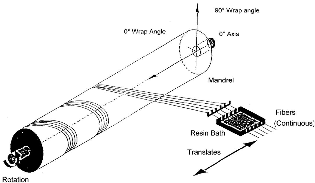
on rotating mandrel. By adjusting the relative speeds of mandrel rotation and glass distribution head movement, helical reinforced pipe is formed. Adjusting the raw materials ratio, which can include high purity silica sand, can also change pipe properties.
