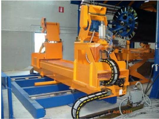
After cutting, the pipe bar is automatically moved away through three lifting tables
